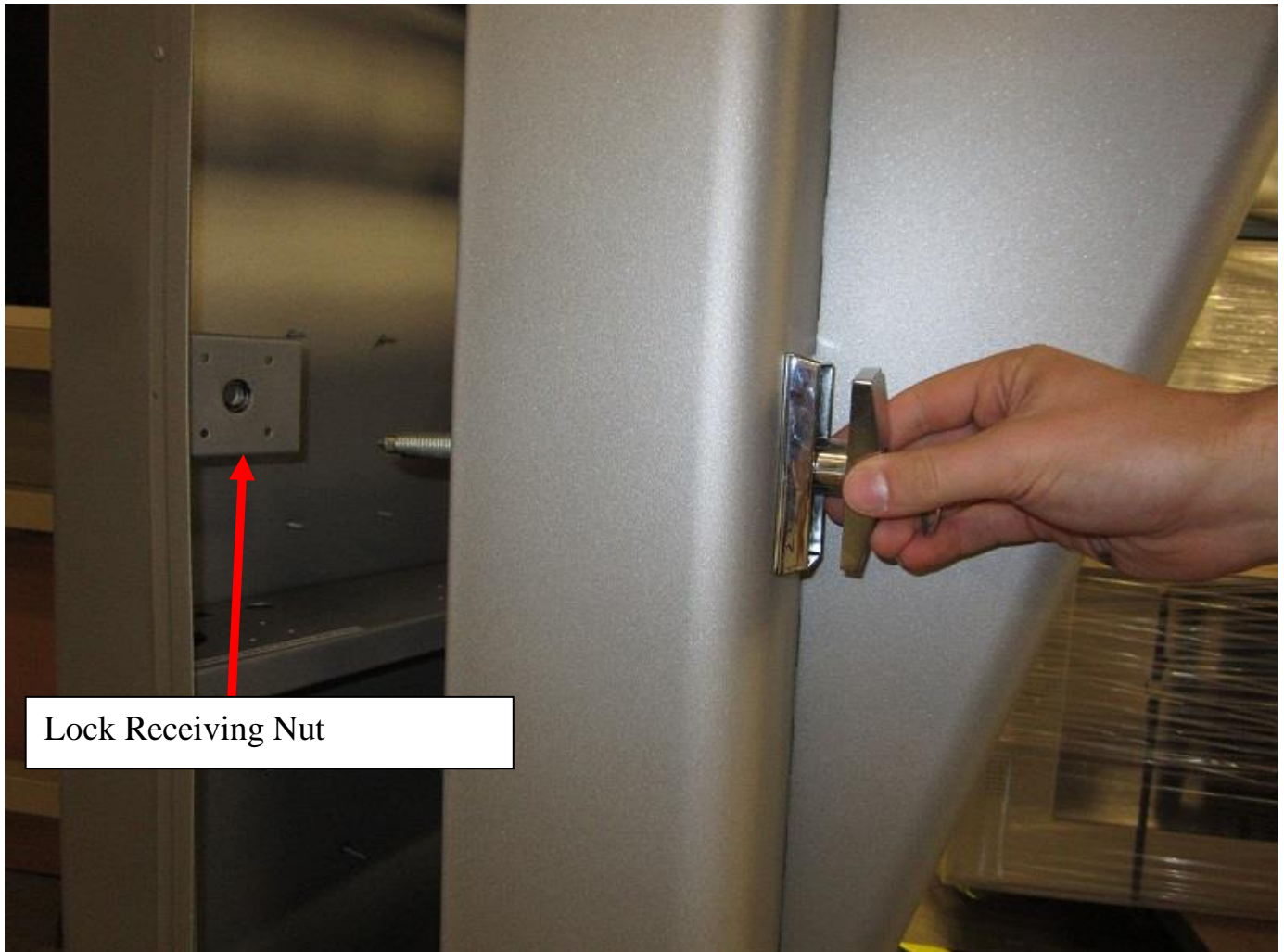
Open (Unscrewed) Lock on Kiosk
