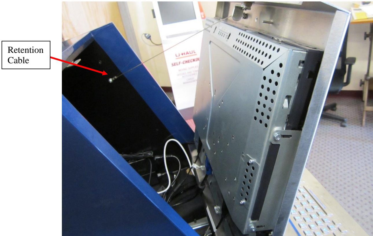
Kiosk with Front Face Open
