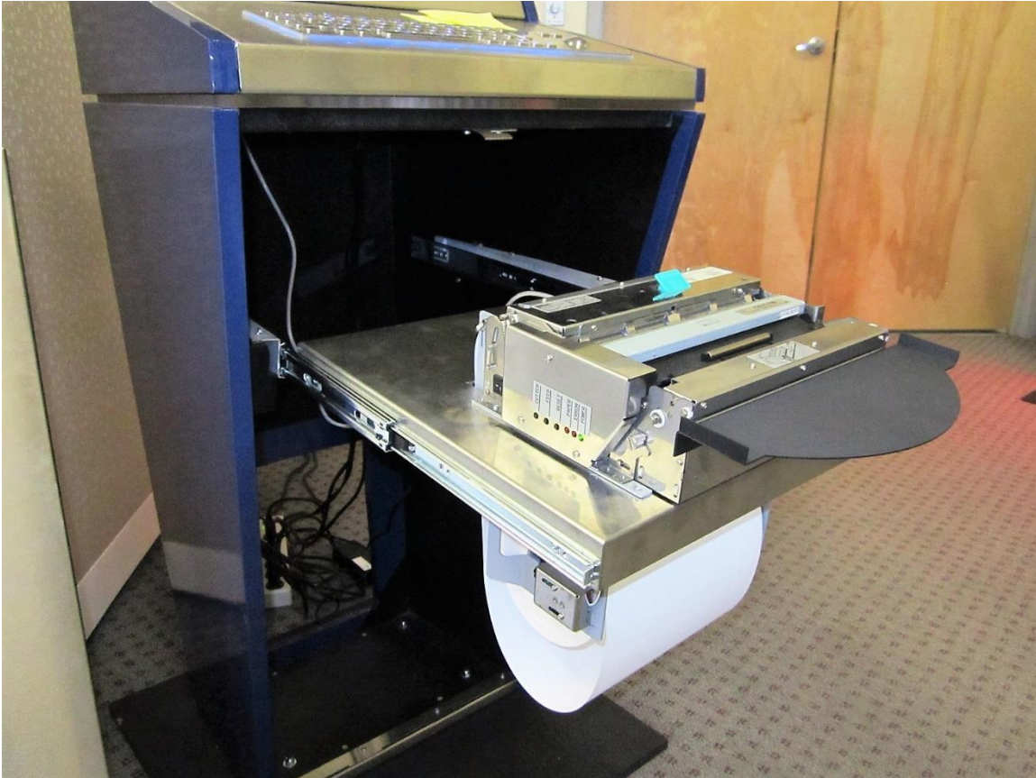
BK-L216II Thermal Printer Mounted to Printer Shelf
