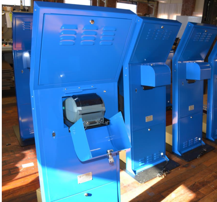
Printer and Shelf Mounted in Kiosk
