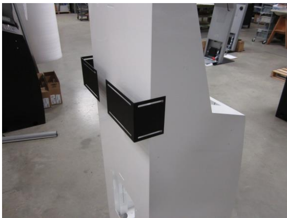
Wall Mounts Facing Inward
